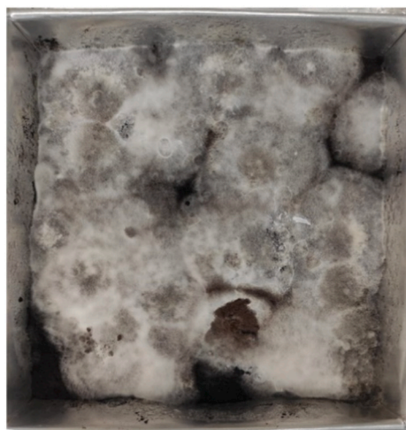
Fig. 14. SCG surface was fully covered with mycelium of P. chrysosporium CK01 during the solid-state fermentation (SSF) process.
